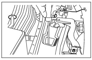
4. Insert a flat blade tool through the opening in the top. Make sure the tool fits through the opening in the headlamp bracket lower arm.
